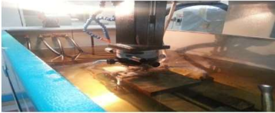
Figure1: Experimental set up of EDM
